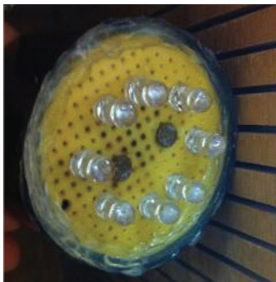
Figure 2: The actual exposure device. The 8 LEDs (each 470 nm) were placed over the plate of cells (Figure 1). The nails heads which served as the source of the magnetic field could be activated singly, the LEDs could be activated singly, or both the field and LEDs could be activated simultaneously
