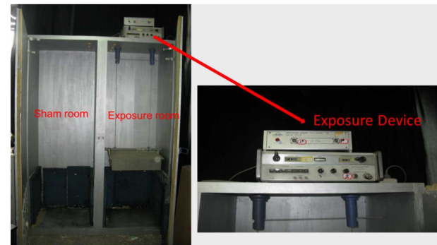
Fig. 1. Exposure devices (length x width x height = 70 x 55 x 200 cm).
