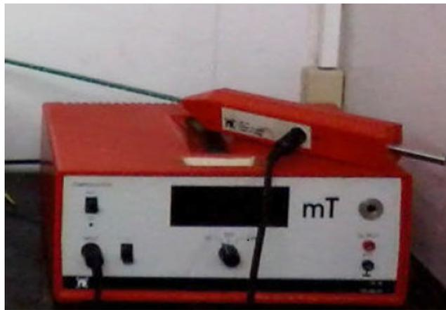
**Figure 3:** Teslameter and its probe
